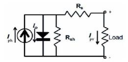
Figure 2: Equivalent Model of a PV Cell
