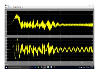
Figure 6: Stator and Rotor Current of Induction Motor
