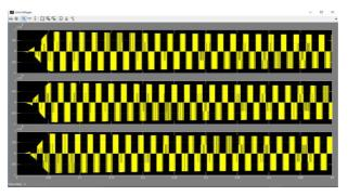
Figure 8: Output of Inverter Showing Line Voltage
