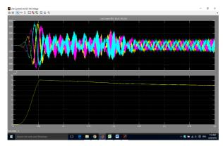
Figure 9: Shows the Three Phase Line Currents and Dc Link Voltage of Inverter
